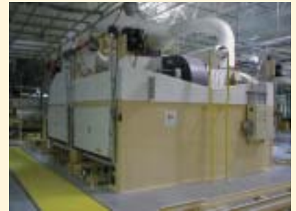
This tightly controlled, high-humidity, low-velocity continuous air dryer enabled a major china manufacturer to increase the speed and efficiency of its drying operation.
